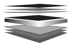
Finish Coat (Nominal 20μm) (Refer Note 4 & 5) Universal Corrosion Inhibitive Primer (Nominal 5μm) Conversion Coating
