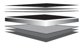
Finish Coat (Nominal 20µm) (Refer Note 4 & 5) Universal Corrosion Inhibitive Primer (Nominal 5µm) Conversion Coating
