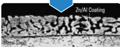
Microscopic view of TRUECORE® steel
