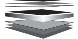
Finish Coat with Antistatic properties (Nominal 20µm) (Refer Note 4 & 5) Corrosion Inhibitive Primer with Antistatic properties (Nominal 5µm) Conversion Coating
