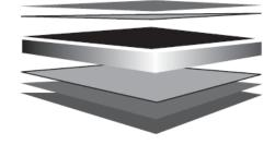
Finish Coat (Nominal 20 $\mu m)$  (Refer Note 4 & 5) Universal Corrosion Inhibitive Primer (Nominal 5 $\mu m)$  Conversion Coating
